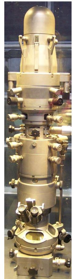
A Scanning Transmission Electron Microscope (STEM) is a specific sort of TEM, where the electrons still pass through the specimen, but, as in SEM, the sample is scanned in a raster fashion.
