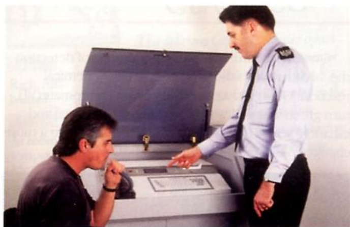
Figure 6 The Lion Intoxilyzer analyses the ethanol in a suspect's breath by absorption of infrared radiation. An immediate print-out of the result is obtained. This is shown to the driver and can be used as evidence in court cases.
